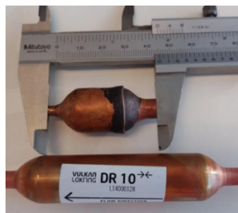
Figure 1: Home-made filter. The picture is of a first trial in which a similar filter with a reduced outlet was modified. In the prototype the filters are of equal overall dimensions but are made by modifying the Vulkan Lokring DR10 filter/drier depicted above.
